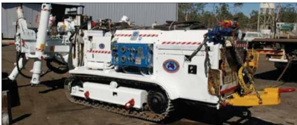
Figure 9.1: Track-mounted Boart Longyear LMC75 drill rig 31
