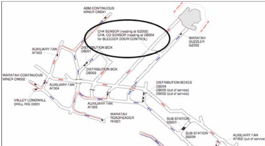
Figure 10.3: Location of hydro-panel sensors 29
