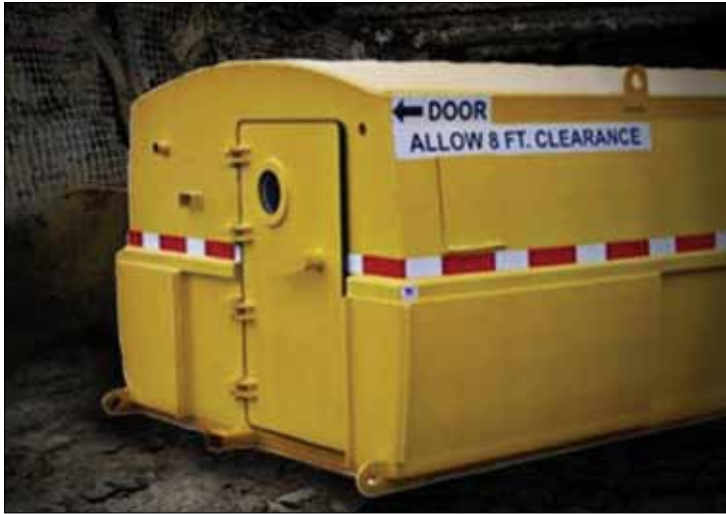
Figure 33.4: Strata Worldwide coal refuge chamber
