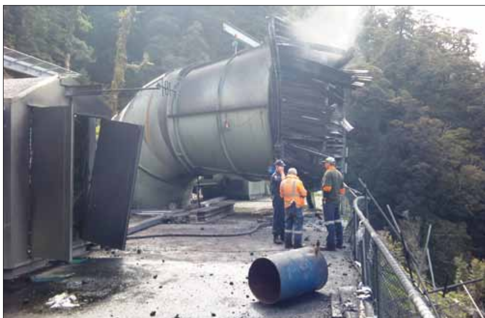
Figure 8.10: The surface fan after the first explosion
