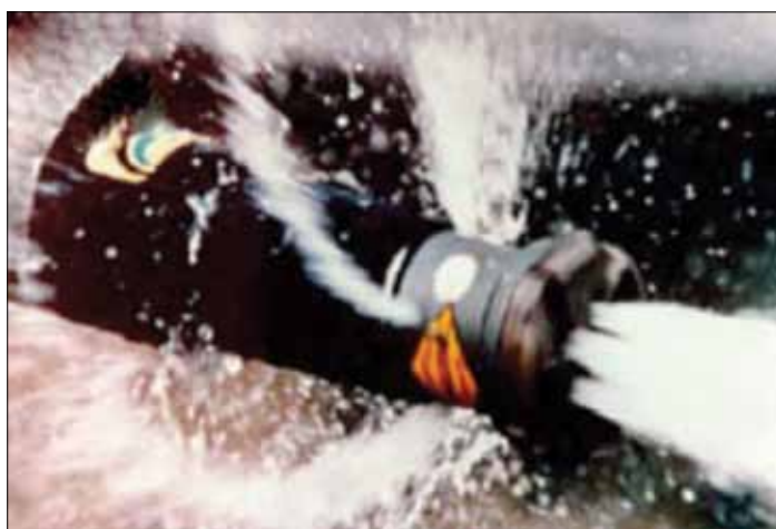
Figure 9.3: Rotating drill bit with high-pressure water 34
