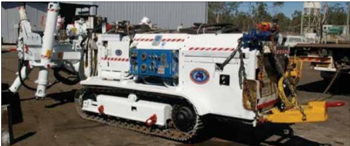
Figure 9.1: Track-mounted Boart Longyear LMC75 drill rig 31
