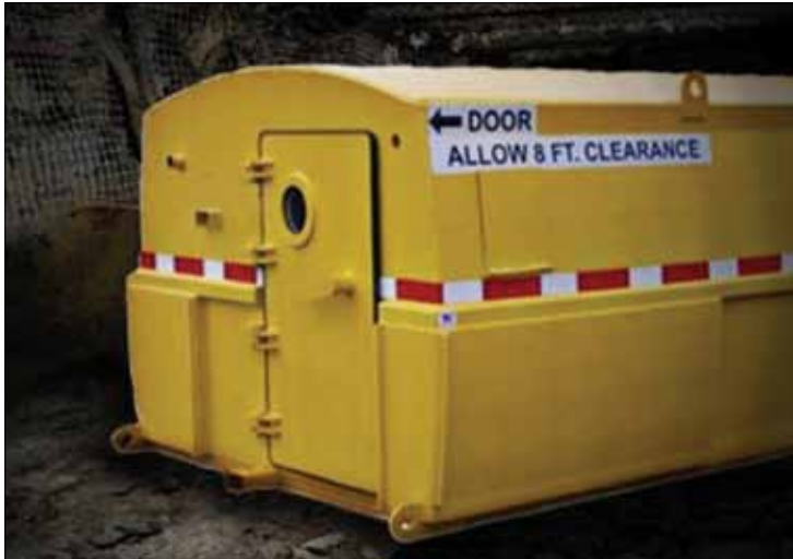
Figure 33.4: Strata Worldwide coal refuge chamber
