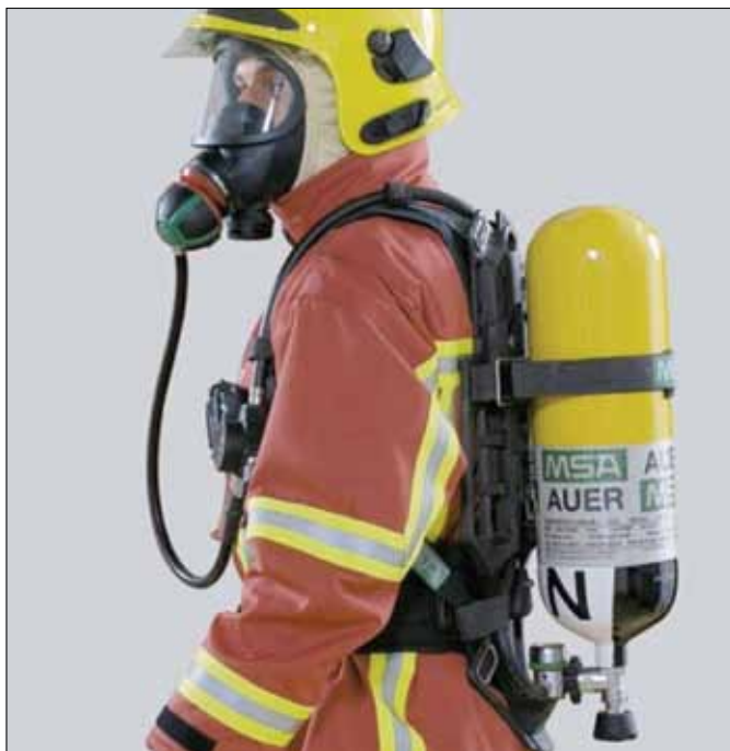
Figure 33.2: Man wearing compressed air breathing apparatus (CABA)
